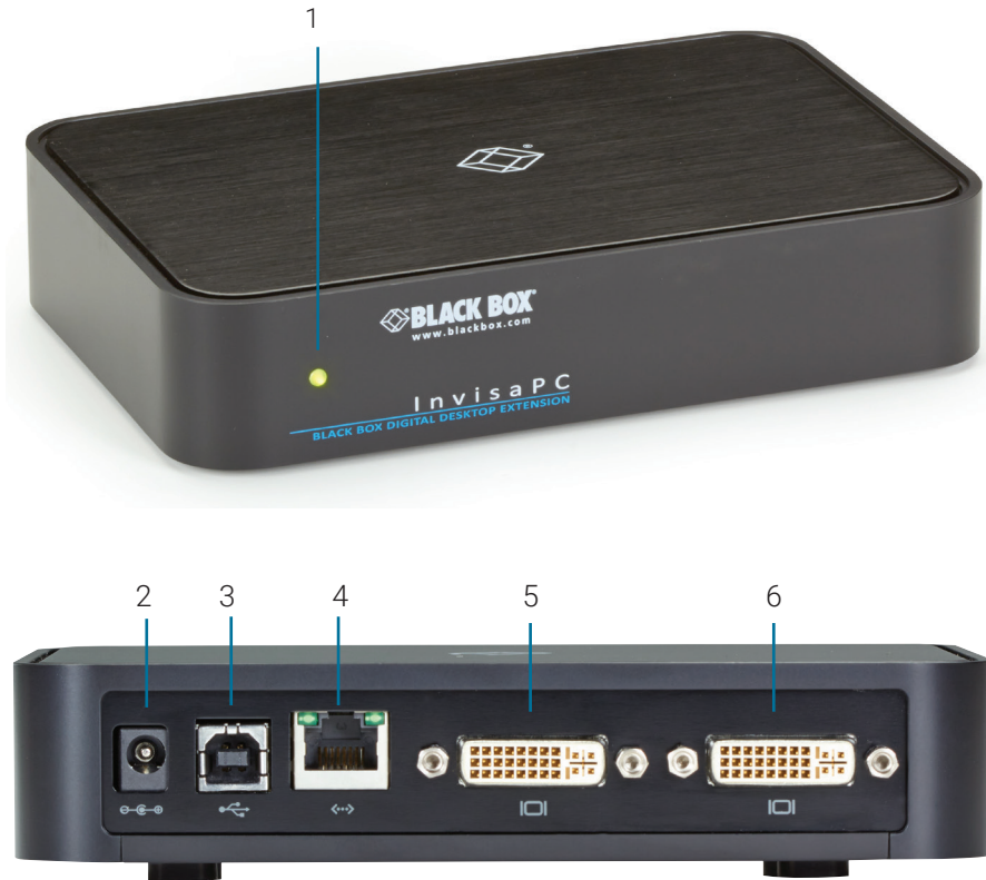
FIGURE 9-2. INVISAPC TRANSMITTER (DTX1002-T) CONNECTIONS
