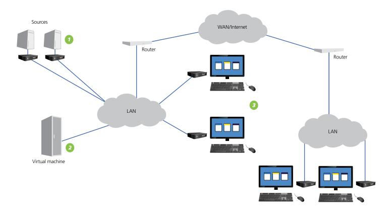
1. InvisaPC transmitters (DTX1000-T) with source CPUs.
