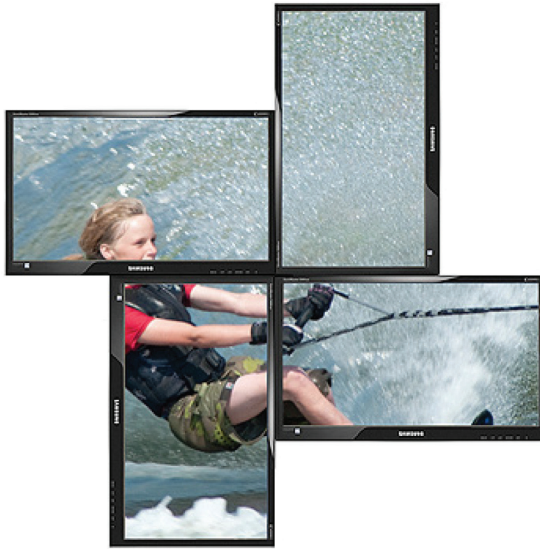
Figure 2-5. Crop the input signal into VideoPlex4 and display x2 quarters landscape and x2 quarters portrait.
