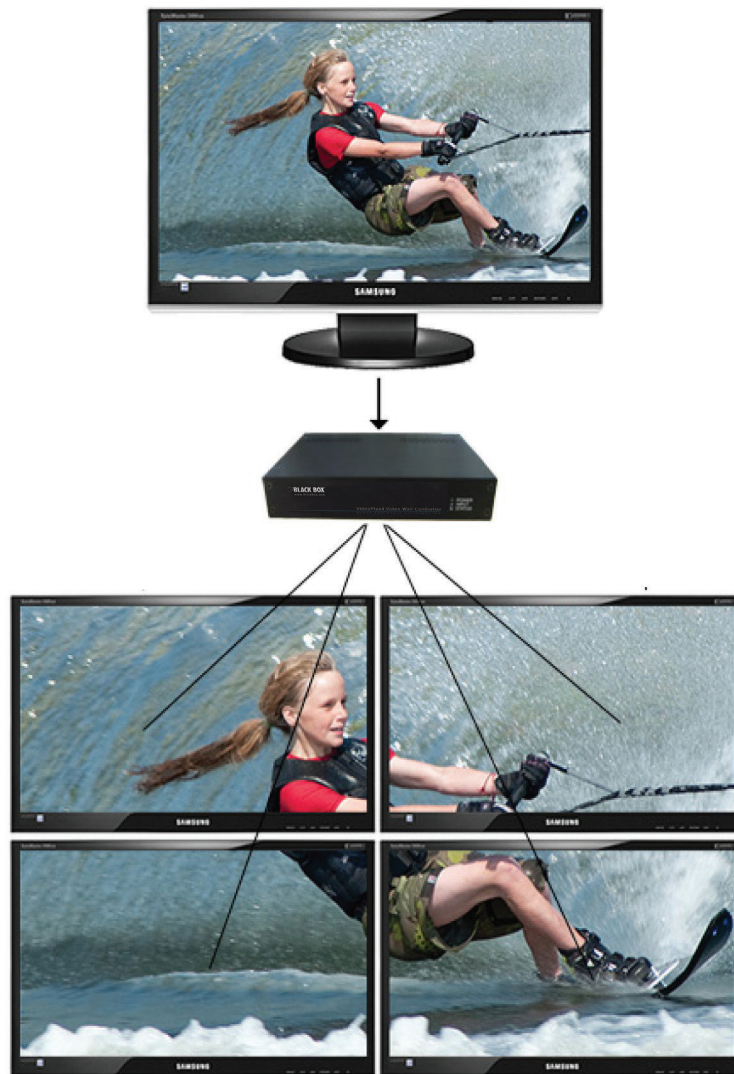
Figure 2-2. Divide the input signal into quadrants and display each quarter on separate displays with optional frame rate conversion (in this case 30 to 60 Hz). You can adjust crop regions to compensate for monitor bezel.
