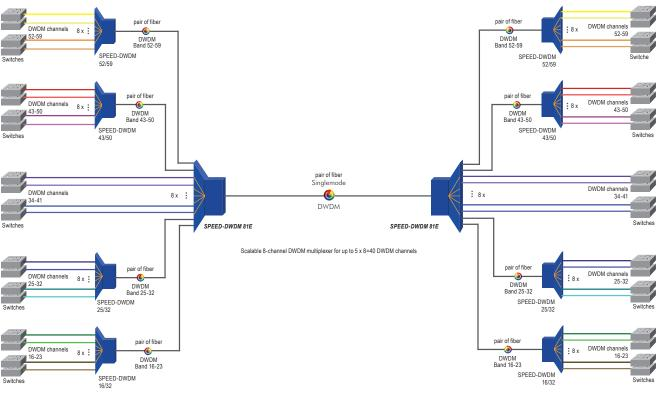
The SPEED-DWDM 81E-34/41-A is a purely passive Mux/Demux module providing 8 DWDM and four extension ports in one unit. In point-to-point connection up to eight applications can be transmitted without additional efforts by using one pair of fibers in a first step. Using the scalable design with four extension ports, further channels can be used for services. Each DWDM channel supports bandwidths from 10
