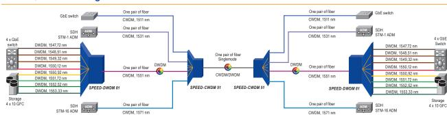
Additionally the SPEED-DWDM 81 can be used for cost-effective upgrading of capacity in existing CWDM networks. The eight wavelengths (1547.72 nm | 1548.51 nm | 1549.32 nm | 1550.12 nm | 1550.92 nm | 1551.72 nm | 1552.52 nm | 1553.33
