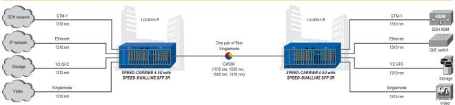
By using the SPEED-DUALLINE SFP 3R it is possible to increase the capacity of one single pair of fiber with a protocol transparent transmission of up to 96 applications (SDH, IP, Storage, video, etc.). The SPEED-DUALLINE SFP 3R performance a conversion of the standard wavelength (850 nm, 1310 nm, 1550 nm) to a dedicated CWDM or DWDM wavelenath an actively managed
