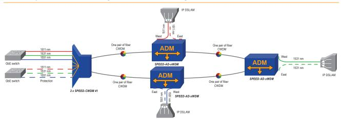
Add/drop multiplexer are often used in ring structures requiring longer distances as constructionconditioned significantly improved attenuation values can be achieved
