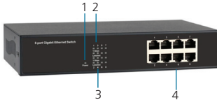
Figure 4-1. LEDs on front panel of switch.
