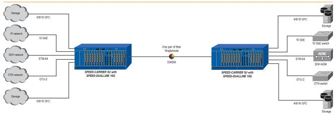
SPEED-DUALLINE 16 G 3R provides a flexible conversion of various protocols, like Ethernet, SDH, OTN und FC to a dedicated CWDM and DWDM wavelenght. Hereby each of the five client ports support a multirate functionality that allows a conversi-
