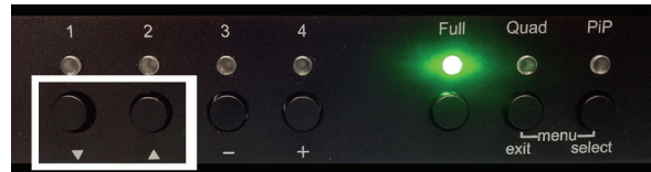
Figure 2-9. Arrow Buttons 1 and 2 enable you to set these resolutions: VGA, SVGA, XGA, and UXGA
