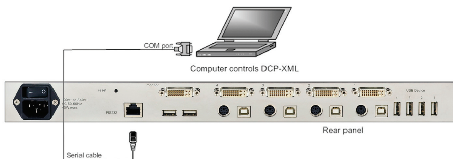
Figure A-5. To update the firmware, connect the computer to the ServSwitch 4site II.
