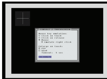
Figure 4-41. The first of four calibration markers appears in the top left corner of the screen. Touch the center of this marker and the other three markers to calibrate the touchscreen.
