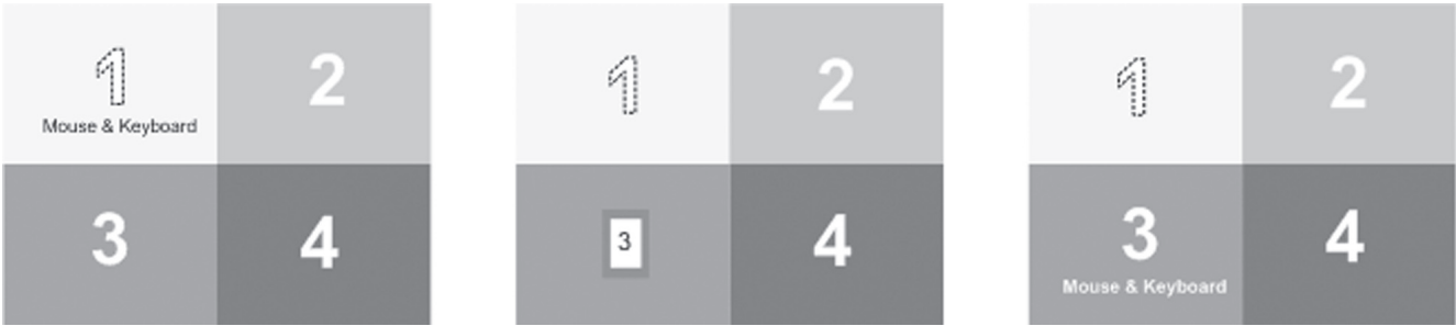
Figure 5-3. This example shows how to switch from Channel 1 to Channel 3.
